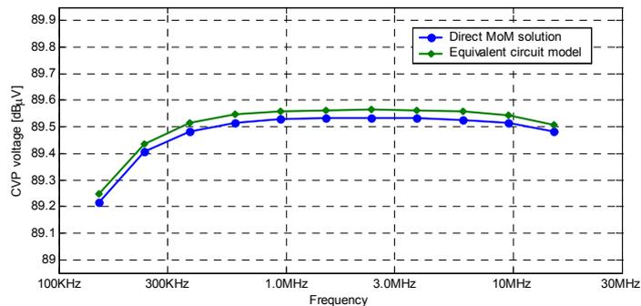
Fig. 5. Voltage coupled in CVP base model. Differing termination loads on cable (50 Ohm and 250 Ohm)
