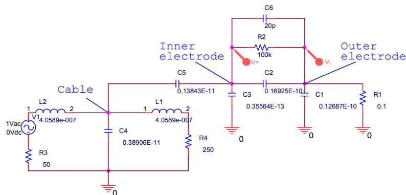
Fig. 3. Equivalent circuit model
