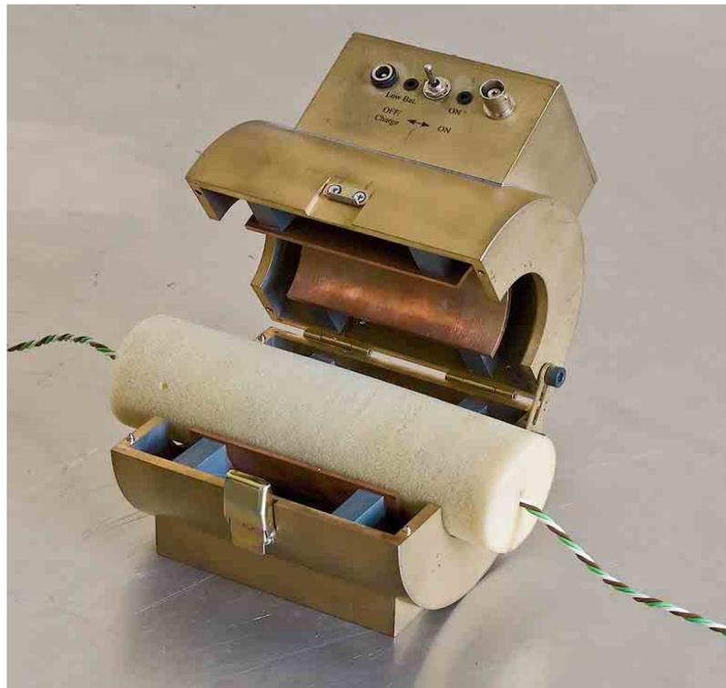
Fig. 1. Capacitive Voltage Probe
