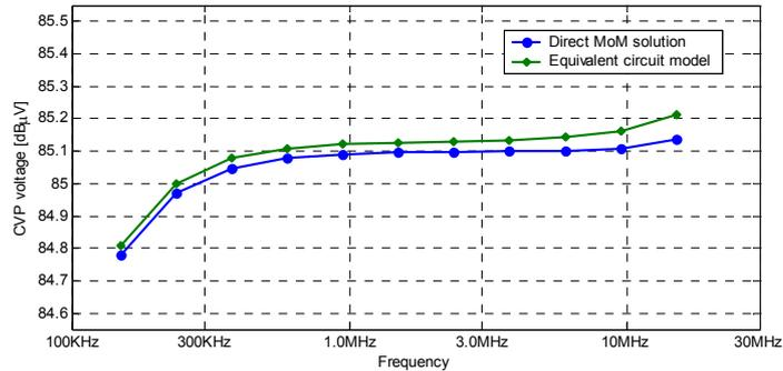
Fig. 4. Voltage coupled in CVP base model. Equal termination loads on cable (50 Ohm and 50 Ohm)
