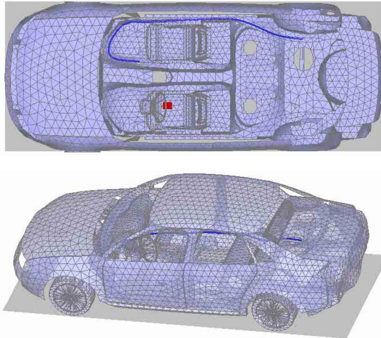
**Fig. 1. Models of ECU and cable, located inside the car**
