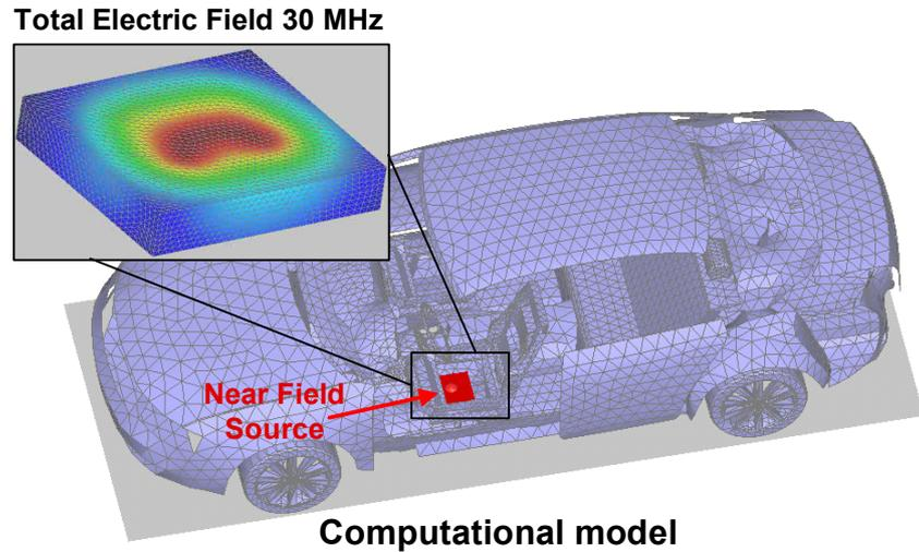
**Fig. 6. Near field source placed in the car**
