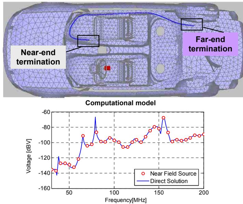
**Fig. 7. Comparison of Near Field Source and direct solution**
