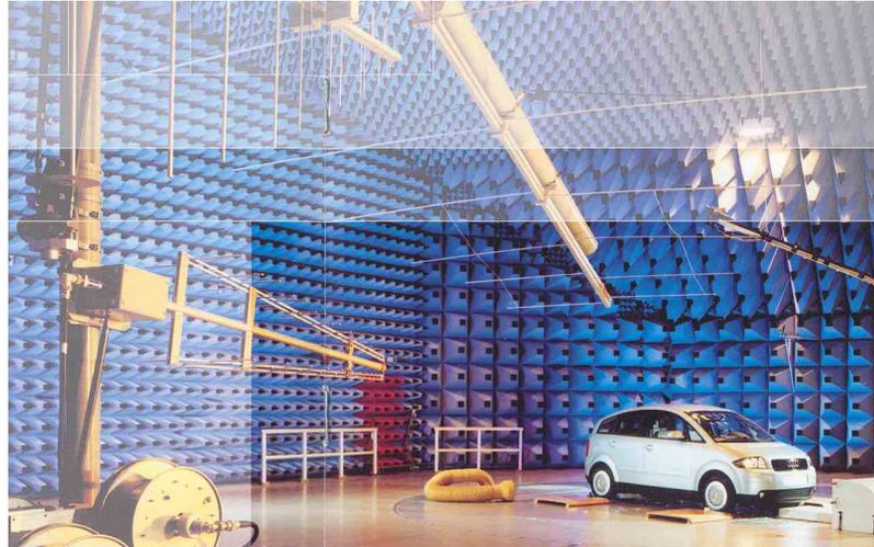
Fig. 1. Anechoic chamber
