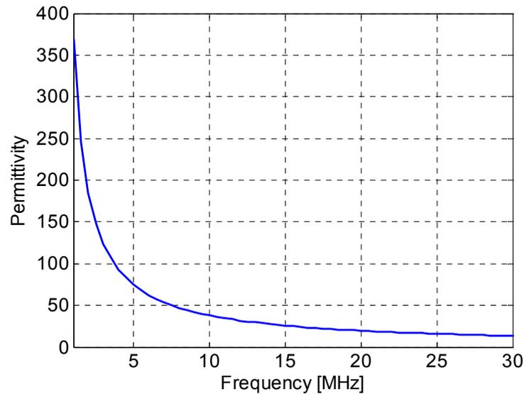
Fig. 4. Frequency dependent permittivity of walls
