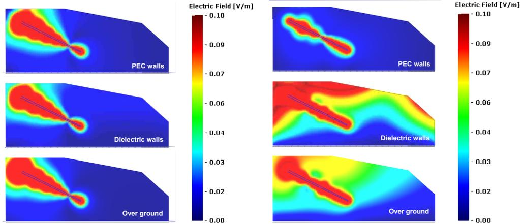
Fig. 7. Electric field at frequency 5 MHz
