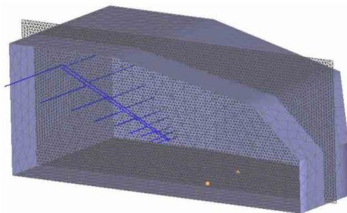
Fig. 2. Log-periodic antenna inside chamber
