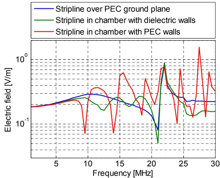
Fig. 6. Electric field produced by stripline in reference point
