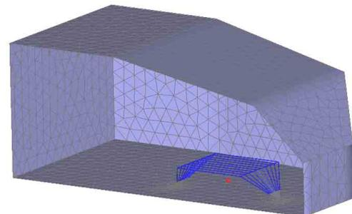
Fig. 3. Radiating stripline inside chamber
