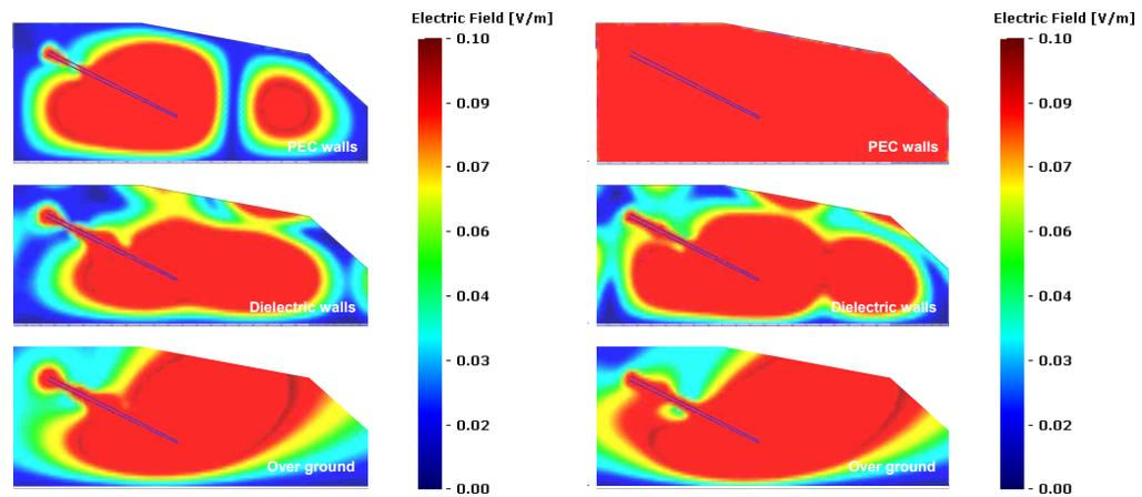
Fig. 9. Electric field at frequency 25 MHz
