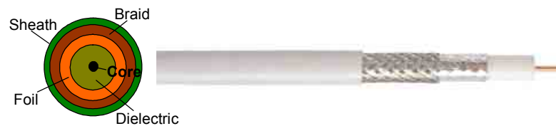
Fig. 1. RG-6/U Type coaxial cable with foil shield and 75% tinned copper braid
