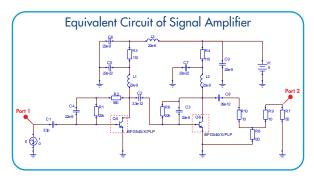
BFG540/X/PLP transistors included in Amplifier circuit are modeled in System Simulation model as Touchstone devices defined from manufacturer's s-parameters datasheet (as \*.snp files).
